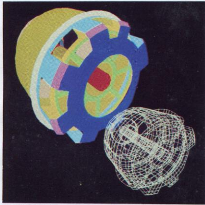
LEX 90's SimulRes enables the designer to mix theory with reality by allowing the simultaneous display of a wireframe model with the real-life product.
